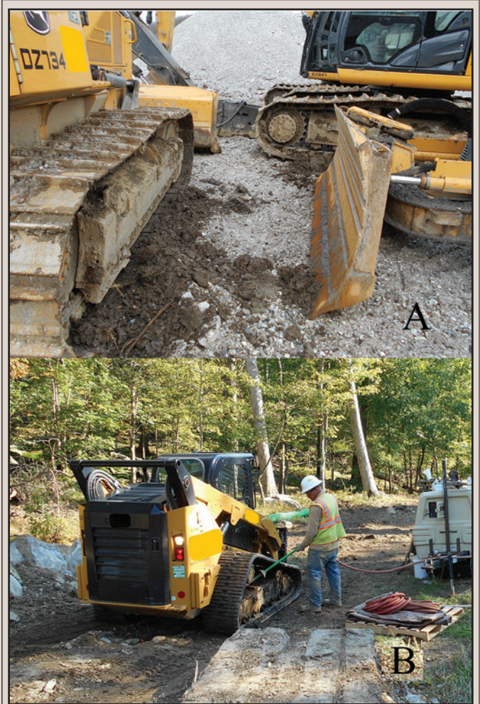
FIG. 3. Cleaning debris from heavy equipment. A) Debris removed from the treads and undercarriage of track-driven equipment. B) Removing debris with pressurized air using an “air spade.”
